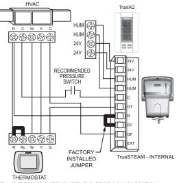
NOTE: IF PRESSURE SWITCH IS USED, ENSURE DIP 5 IS IN ON POSITION. M27341
